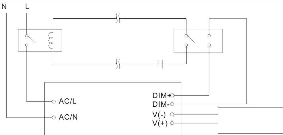
by using a switch and a relay, you can turn on and off the lighting device.
